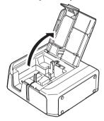
3. Place a tape cartridge in the printer as shown.
