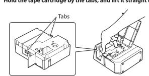
3. Place a new tape cartridge in the printer.
